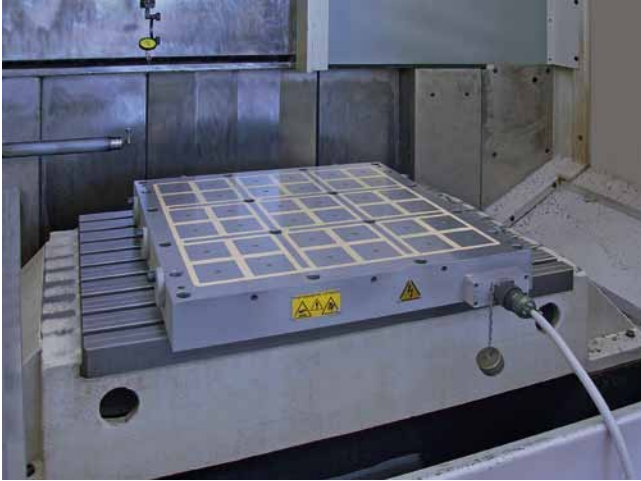
Magnetic clamping plate with square poles 70 x 70, plate size 630 x 630 mm, with laterally drilled holes for stop bars
