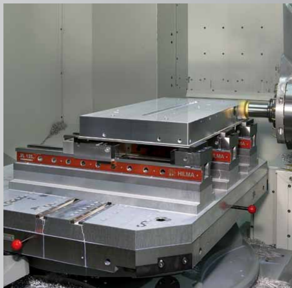
Clamping of plate-shaped workpieces requiring heavy machining.
