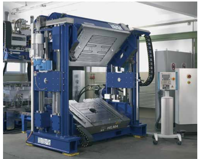
Magnetic clamping system for a mould carrier 1500 x 1000 mm, retaining force 200 kN; temperature range up to 120°C.
