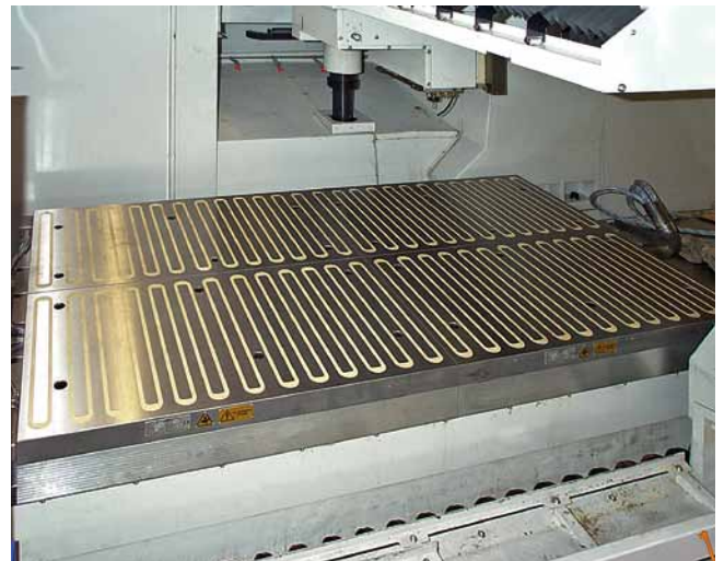
M-TECS long LP poles with power concentration for very small moulds and special applications
