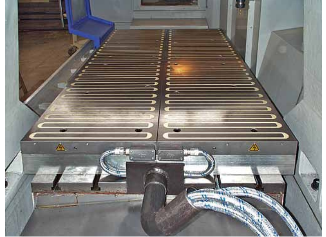
Long poles for heavy machining, plate size 2200 x 1200 mm, with 2 connections. Magnetic retaining force 800 kN.
