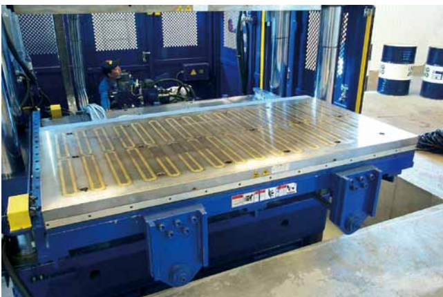
Magnetic clamping system for a sliding table 2500 x 1200 mm, retaining force 800 kN, temperature range up to 230°C.
