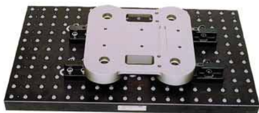
Down draw clamp for pegging out zero point
