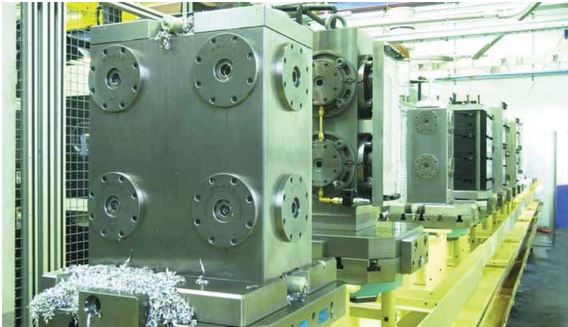
Mounting towers with SPEEDY 1000 and SPEEDY 1000 assembly with pipe system.
