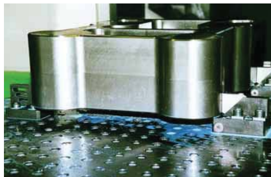
Finished work piece clamped with down draw clamp, raised model
