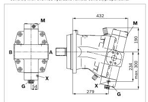
▼ EP.D, EP.G – Proportional control electric, with pressure control fixed setting; remote controlled (EP.G)
