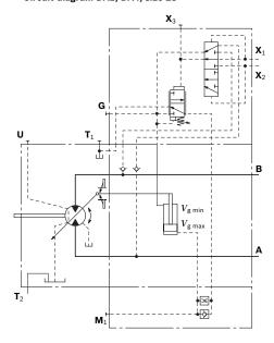
Axial piston variable motor | **A6VM Series 63**DA – Automatic control, speed related
