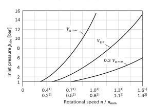
This diagram is only valid for the optimum viscosity range of  $\nu_{\text{opt}}$  = 36 to 16 mm²/s.
