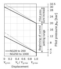
Axial piston variable motor | **A6VM Series 63** HD – Proportional control, hydraulic
