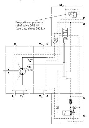
Axial piston variable motor | **A6VM Series 63** EP – Proportional control, electric 17
