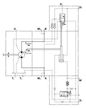
A6VM Series 63 | Axial piston variable motor EP - Proportional control, electric
