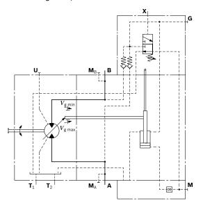
20 A6VM Series 63 | Axial piston variable motor EZ – Two-point control, electric
