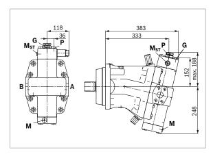
▼ EP.D, EP.G – Proportional control electric, with pressure control fixed setting; remote controlled (EP.G)
