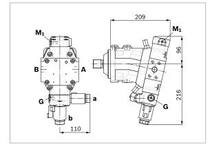
▼ DA2, DA3, DA5, DA6 – Automatic speed related control, with electric travel direction valve and electric  $V_{\rm g\ max}$ -circuit
