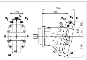
88 A6VM Series 63 | Axial piston variable motor Dimensions, sizes 355 Dimensions [mm]
