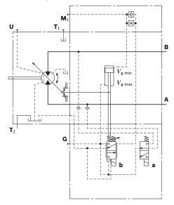
28 A6VM Series 63 | Axial piston variable motor DA – Automatic control, speed related
