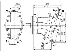
HD.D, HD.G - Proportional control hydraulic with pressure control fixed setting; remote controlled (HD.G)
