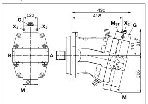
44 **A6VM Series 63** | Axial piston variable motor Dimensions, sizes 1000
