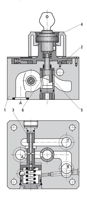
The flow control valve type 3FRM is a 3-way flow control valve. It is used for maintaining a set constant flow, independent of changes in pressure and temperature. The valve basically consists of a housing (1), an orifice bush (2), a pressure compensator (3) and an adjustment type (4).
