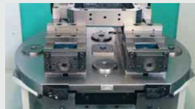
Square SPEEDY classic 1 STANDARD for single mounting (positioned secured against turning)
