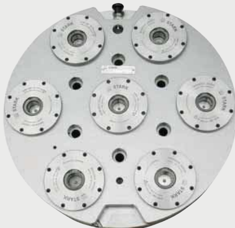
SPEEDY classic 2 STANDARD round fitted in plate with matched fastening and positioning bores.
