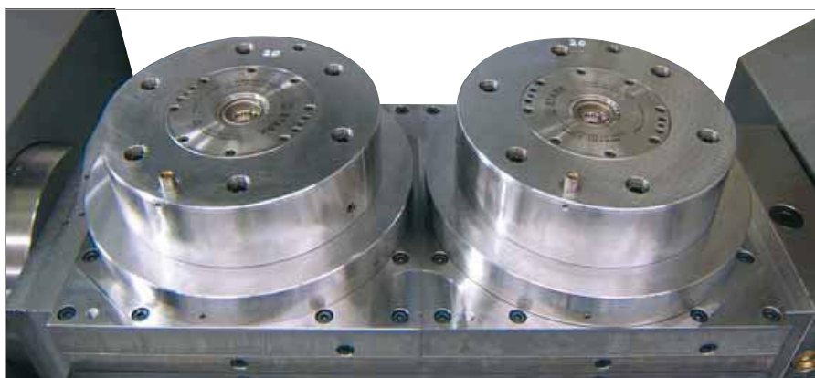
SPEEDY classic 2 with two integrated media ducts, fitted to swivelling yoke.
