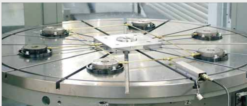
SPEEDY classic 2 Surface Mount with hydraulic pipework
