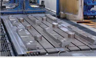
SPEEDY classic 3 fast closing clamps fitted in clamping strips with pipework. Using the two jigs,
