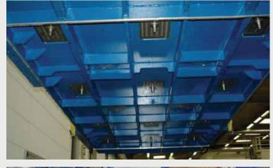
Machine pallet with clamping device for workpieces.
