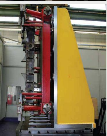
Clamping angle for workpieces up to 2.5 m high with 12 SPEEDY classic 3, 360 kN insertion force.
