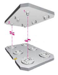
**Application:** Equalisation of thermal expansion and manufacturing tolerances.
