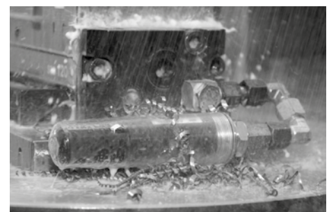
10 pressure sensors with radio transmission
