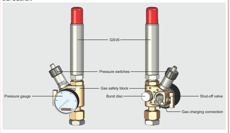
The gas safety block GSB450 consists of a brass block (other materials on request) with an integrated vent valve and shut-off valve and connections for:
