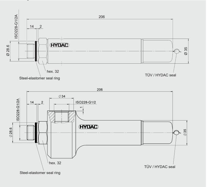
Selection of the response pressure (p) of the gas safety valve is based on the maximum operating pressure of the hydraulic accumulator, according to the application.
