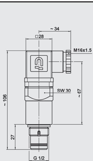
\* The clogging indicator is simple electrical operating equipment according to DIN EN 60079-14 and may only be used in intrinsically safe circuits (supplied with manufacturer's declaration and operating instructions).
