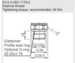
With temperature measurement as an option: G1/2 A ISO 1179-2 with measurement probe External thread tightening torque, recommended: 45 Nm
