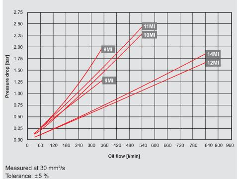
For other viscosities, the pressure loss must be multiplied by the conversion factor K:
