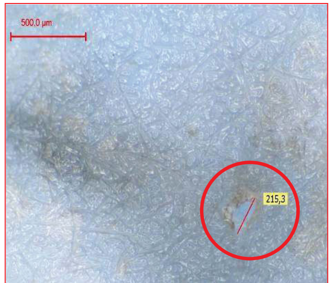
Burn hole in the filter material
