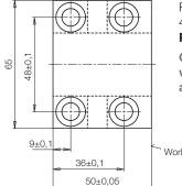
Fixing screws 4x M8x25 12.9
