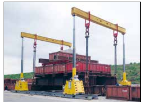
SL400 Gantry during load testing. ►
