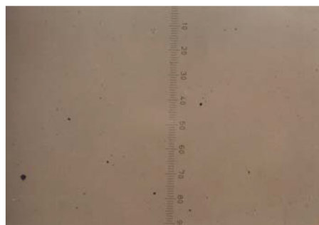
Fig. 11 Microscopic Examination of an Oil Sample (100 ml) Magnification 100x (ISO 18 / 15 / 11)
