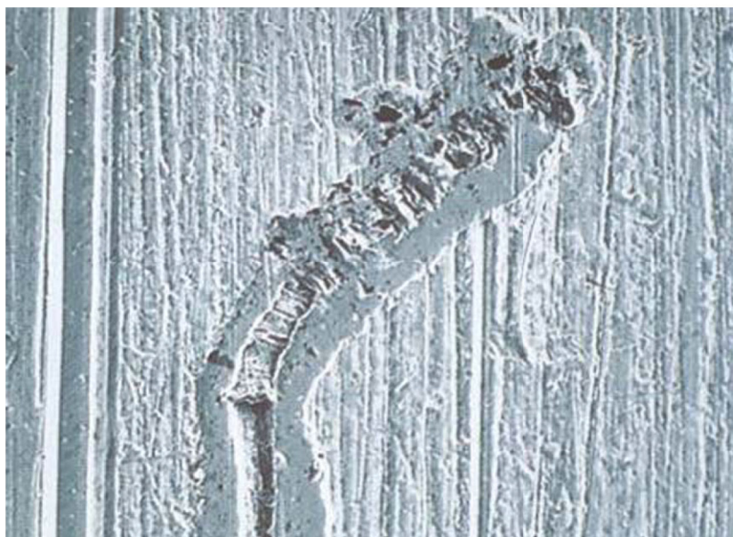
Fig. 9 Chip Embedded in the Surface of a Friction Bearing
