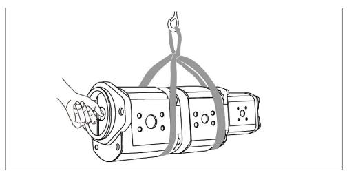
Fig. 5: Transport with lifting strap
