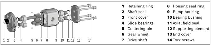
Fig. 3: External gear pump layout
