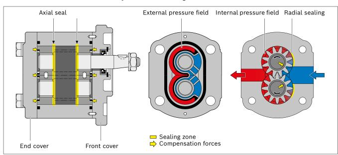
Fig. 2: Axial compensation external gear pump
