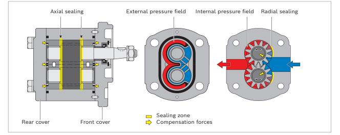
Axial and radial sealing of gear chambers
