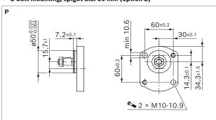
4-bolt mounting, spigot dia. 52 mm, with O-ring
