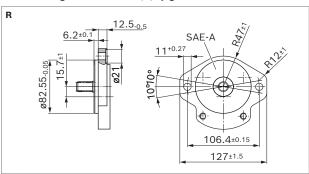
2-bolt flange SAE J744 101-2 (B) spigot dia. 101.6 mm
