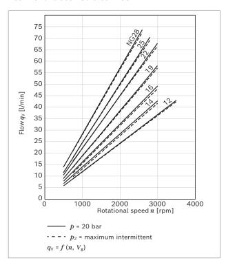
▶ Characteristic curves measured at  $v = 32 \text{ mm}^2/\text{s}$  and *t* = 50 °C
