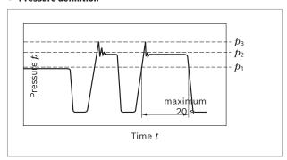
p<sub>1</sub>: Maximum continuous pressurep<sub>2</sub>: Maximum intermittent pressure
