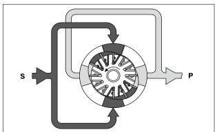
Hydraulic pumps of type PVH are vane pumps with fixed displacement volume.
