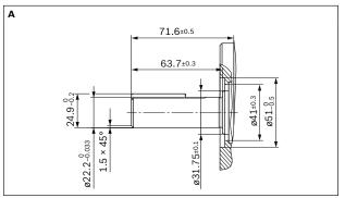
$_{\rm 1)}$  Involute spline according to ANSI B92.1a, 30° pressure angle, flat root, side fit, tolerance class 5
