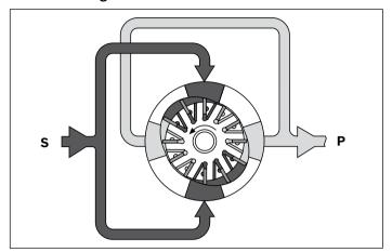
Hydraulic pumps of type PVH are vane pumps with fixed displacement volume.
