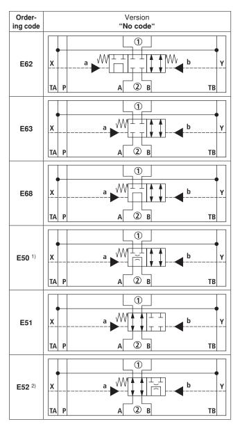
$<sup>^{1)}</sup>$  Opening cross-section in spool position "a" (A2  $\rightarrow$  B2) = 50  $\text{mm}^2$
