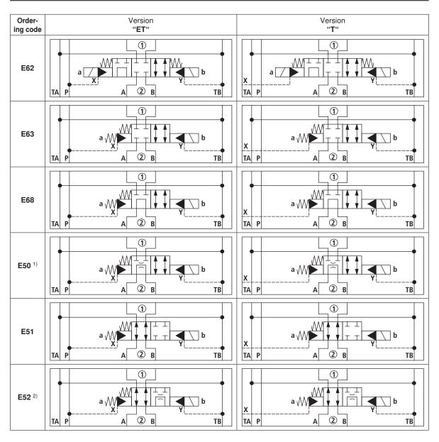
$<sup>^{1)}</sup>$  Opening cross-section in spool position "a" (A2  $\rightarrow$  B2) = 50  $\text{mm}^2$
