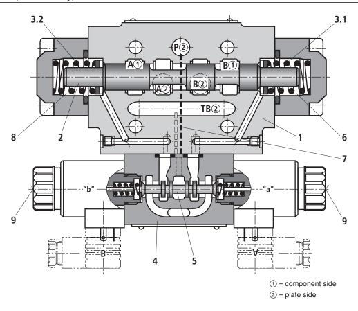
Valves of type Z4WEH are directional spool valves with electrohydraulic actuation. They control the start and stop of a flow.
