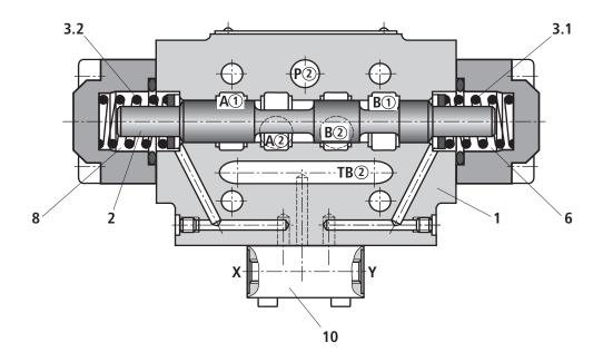
Valves of type Z4WH are directional spool valves with hydraulic actuation. They control the start and stop of a flow.
