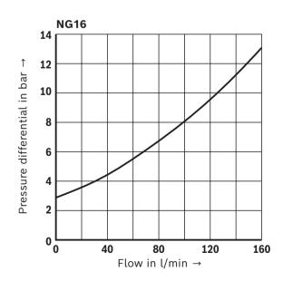
**Characteristic curves:** 2-way flow control valve (measured with HLP46,  $\vartheta_{oil}$  = 40 ±5 °C)
