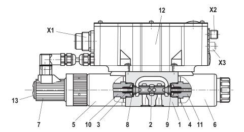
**Notice!** The PG fitting (13) must not be opened. Mechanical adjustment of the adjustment nut located below is prohibited and damages the valve!
