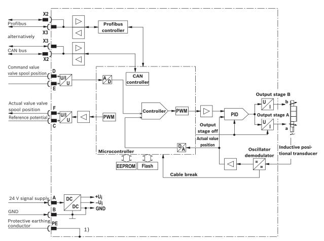
1) The protective earthing conductor (PE) is connected to cooling element and valve housing.
