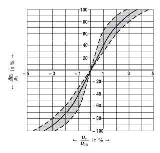
**Zero flow** (with central control spool position - V control spool)
