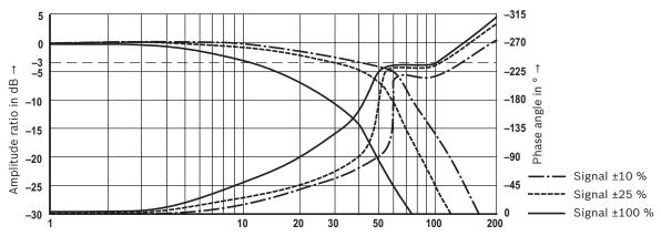
Pressure/signal characteristic curve (V control spool),
