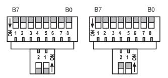
Connection of the bus terminator with the two lower switches (only with PROFIBUS-DP):
