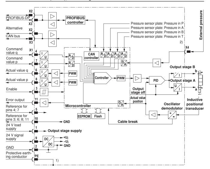
Command value: Positive command value 0 to +10 V (or 12 to 20 mA) at pin 4 and reference potential at pin 5 result in
