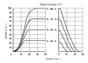
Frequency response characteristic curves: Size 6 (measured using HLP46,  $\theta_{\rm oil}$  = 40 °C ±5 °C,  $\rho_{\rm s}$  = 10 bar)
