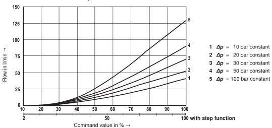
$\Delta p$  = valve pressure differential (inlet pressure  $p_P$  minus load pressure  $p_L$  minus return flow pressure  $p_T$ )
