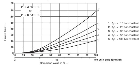
50 I/min rated flow at 10 bar valve pressure differential
