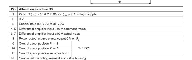
Command value: Positive command value 0 to +10 V at pin 4 and reference potential at pin 5 result in flow from P  $\rightarrow$  A and B  $\rightarrow$  T.
