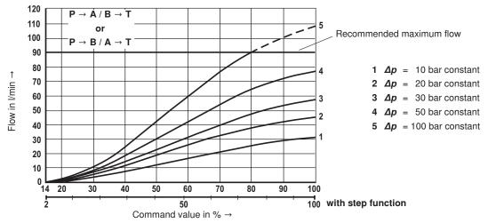
$\Delta p$  = valve pressure differential (inlet pressure  $p_P$  minus load pressure  $p_L$  minus return flow pressure  $p_T$ )
