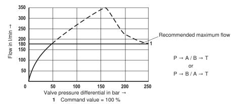
Transition function with stepped electric input signals: Size 10
