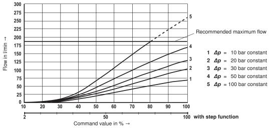
$\Delta p$  = valve pressure differential (inlet pressure  $p_P$  minus load pressure  $p_T$  minus return flow pressure  $p_T$ )
