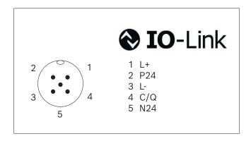
Fig. 4: Name plate of IO-Link electronics
