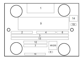
Fig. 3: Name plate of valve 4WRPEH6
