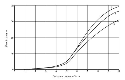
Characteristic curves measured with directional control valve type 4WRPE 6 ...
