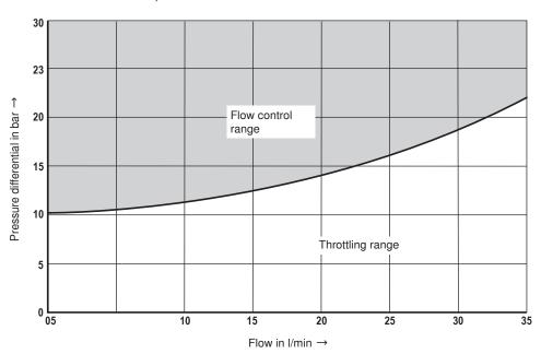
Pressure differential  $\Delta \boldsymbol{p}_{\min} = \boldsymbol{p}_{\text{Pump}} - \boldsymbol{p}_{\text{Load}}$
