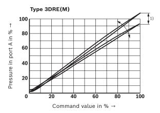
1) In order to be able to adjust several valves to the same characteristic curve, the manufacturing tolerance can - with version 3DRE(M) - be changed at the external amplifier (see page 18) using the command value attenuator "G". In this connection, do not set the pressure higher than the maximum set pressure of the pressure rating with command value 100 %.
