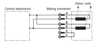
The coils are connected in parallel in the mating connector or on the amplifier (see figure).
