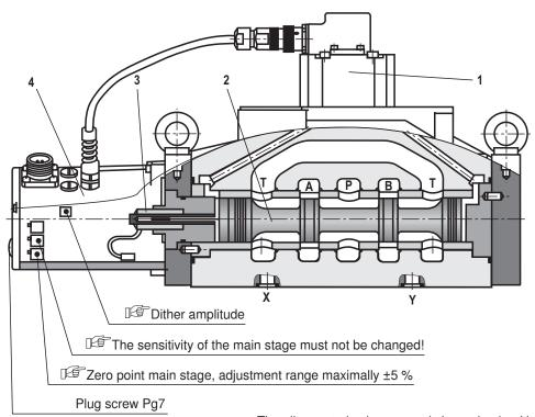
The pilot control valve may only be maintained by Bosch Rexroth employees. An exception to this is the replacement of the filter element – see data sheet 29564.
