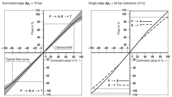
\* With interface F1, the negative command value axis corresponds to 4 to 12 mA, the positive command value axis to 12 to 20 mA
