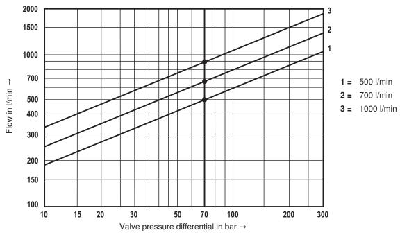
$\Delta p$  = Valve pressure differential (inlet pressure  $p_P$  minus load pressure  $p_L$  minus return flow pressure  $p_T$ )
