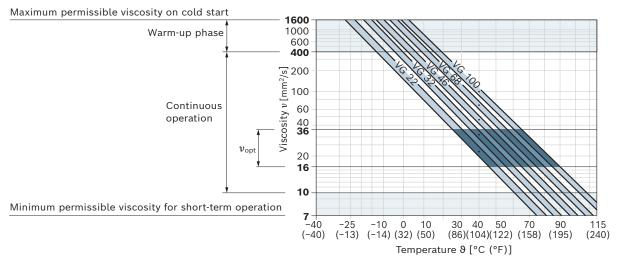
$<sup>^{1)}</sup>$  This corresponds, for example on the VG 46, to a temperature range of +4 °C (+39 °F) to +85 °C (+185 °F) (see selection diagram)
