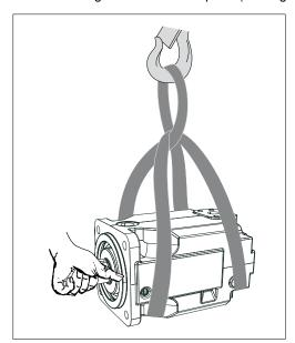
Fig. 5: Transport with lifting strap
