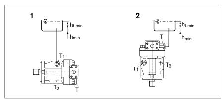
Fig. 6: Below-reservoir installation for size 22 to 56 with installation position 1-2
