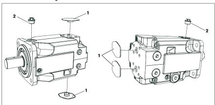
Fig. 1: Axial piston unit
