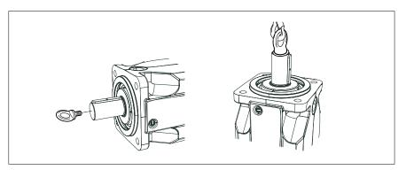
Fig. 4: Fixing the ring screw
