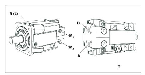
Fig. 13: Port overview A4FM, size 71, SAE flange ports at back (port plate 01)
