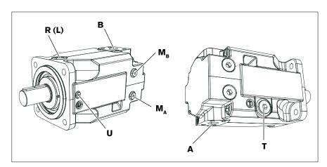
Fig. 14: Port overview A4FM, size 125 to 500, SAE flange ports on opposite sides (port plate 02)
