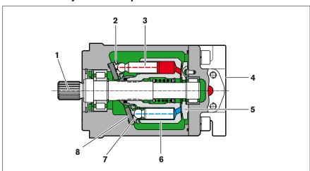
Fig. 2: Assembly of the A4FM
