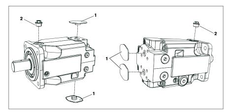
Fig. 11: Removing transport protection
