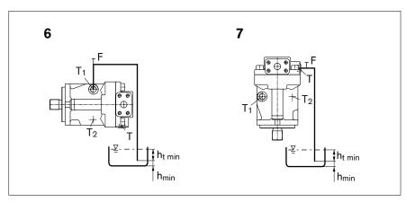
Fig. 8: Above-reservoir installation for size 22 to 56 with installation position 6-7
