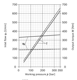
*n* = 2600 rpm *n* = 1500 rpm
