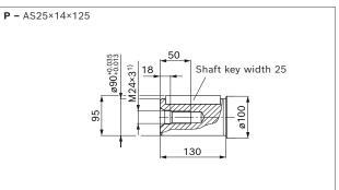
1) Center bore according to DIN 332 (thread according to DIN 13)
