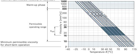
$_{\rm 1}$  This corresponds, for example on the VG 46, to a temperature range of +4 °C to +85 °C (see selection diagram)
