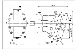
▼ **EP.D, EP.G** – Proportional control, electric, with fixed pressure control setting; remote controlled (EP.G)
