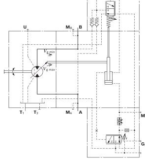
Axial piston variable motor | **A6VM series 63** 13 HD – Proportional control, hydraulic
