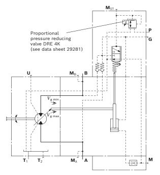
Axial piston variable motor | **A6VM series 63** 15 EP – Proportional control, electric
