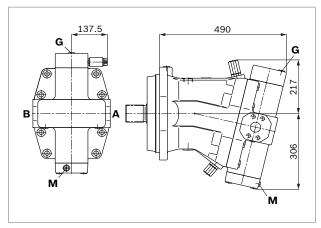
DA – Automatic control, speed related, with hydraulic travel direction valve
