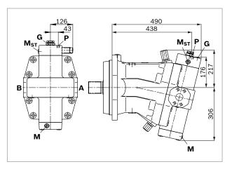
HD.D, HD.G – Proportional control, hydraulic, with fixed pressure control setting; remote controlled (HD.G)
