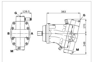
▼ DA - Automatic control, speed related, with hydraulic travel direction valve
