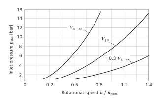
Minimum pressure – operation as a pump (inlet)
