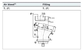
1) Because complete air bleeding and filling are not possible in this position, the motor should be air bled and filled in a horizontal position before installation.
