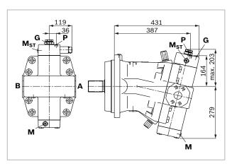
HD.D, HD.G – Proportional control, hydraulic, with fixed pressure control setting; remote controlled (HD.G)
