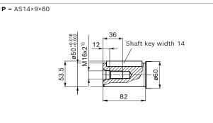
1) Center bore according to DIN 332 (thread according to DIN 13)
