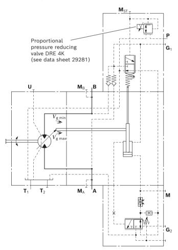
Pressure control with 2nd pressure setting is available as standard with EP.D control.
