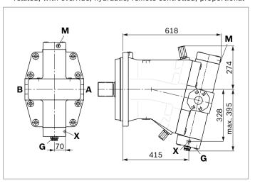
▼ **EP.D, EP.G** – Proportional control, electric, with fixed pressure control setting; remote controlled (EP.G)
