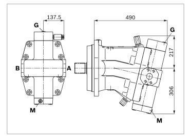
▼ DA - Automatic control, speed related, with hydraulic travel direction valve
