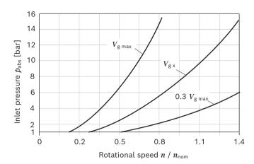
This diagram is only valid for the optimum viscosity range of  $\nu_{\text{opt}}$  = 36 to 16 mm²/s.
