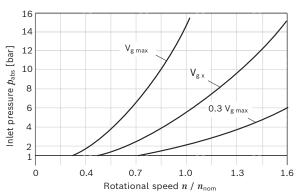
This diagram is valid only for the optimum viscosity range from  $v_{\text{opt}}$  = 36 to 16  $\text{mm}^2/\text{s}.$
