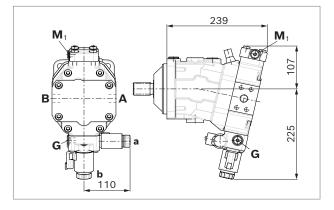
Port plate 1 - SAE working ports **A** and **B** at rear
