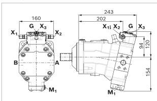
$\mathbf{X}_1$ ,  $\mathbf{X}_2$  Pipe fitting SDSC – L8×M12 – F acc. to ISO 8434-1 Use assembled fitting!
