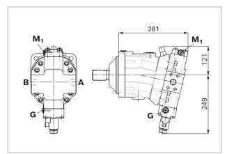
▼ EP5D1, EP6D1 - Proportional electric control, negative control, with pressure control fixed setting
