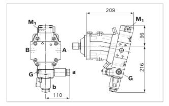
f V DA1, DA2 – Automatic speed related control, negative control, with electric travel direction valve and electric  $V_{\rm g\,max}$  override
