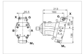
▼ **HP5D1, HP6D1** – Proportional hydraulic control, negative control, with pressure control fixed setting
