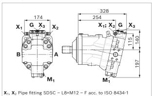
▼ DA1, DA2 - Automatic speed related control, negative control, with electric travel direction valve and electric V<sub>g max</sub> override
