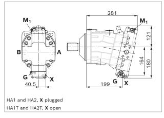
▼ HA1R1, HA2R2 - Automatic high-pressure related control, positive control, with electric override and electric travel direction valve
