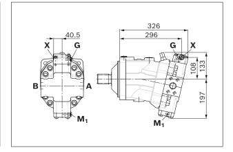
▼ HP5D1, HP6D1 - Proportional hydraulic control, negative control, with pressure control fixed setting
