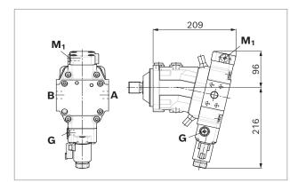
▼ DA0 - Automatic speed related control, negative control, with hydraulic travel direction valve
