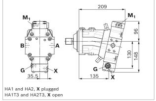
▼ HA1R1, HA2R2 – Automatic high-pressure related control, positive control, with electric override and electric travel direction valve
