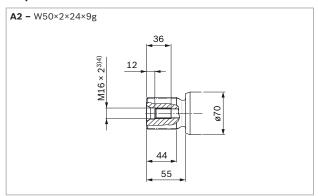
$_{\rm 1)}$  Involute spline according to ANSI B92.1a, 30° pressure angle, flat root, side fit, tolerance class 5
