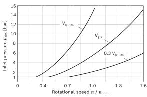
This diagram is valid only for the optimum viscosity range from  $v_{\text{opt}}$  = 36 to 16 mm²/s.
