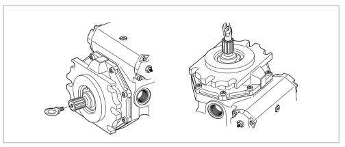
Fig. 5: Fixing the eye bolt
