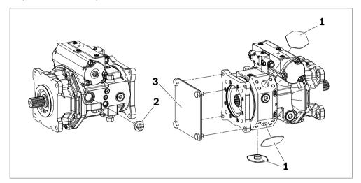
Fig. 11: Removing transport protection
