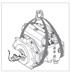
Fig. 6: Transport with lifting strap
