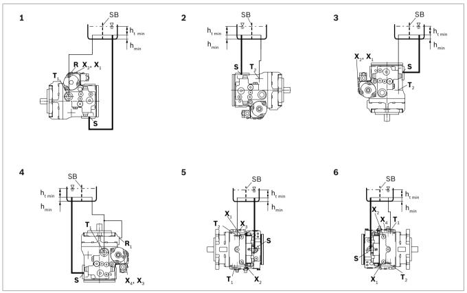
Fig. 8: Below-reservoir installation with installation position 1-6
