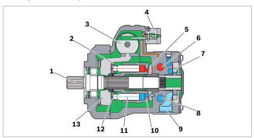
Fig. 2: Layout of the A4VG Series 40
