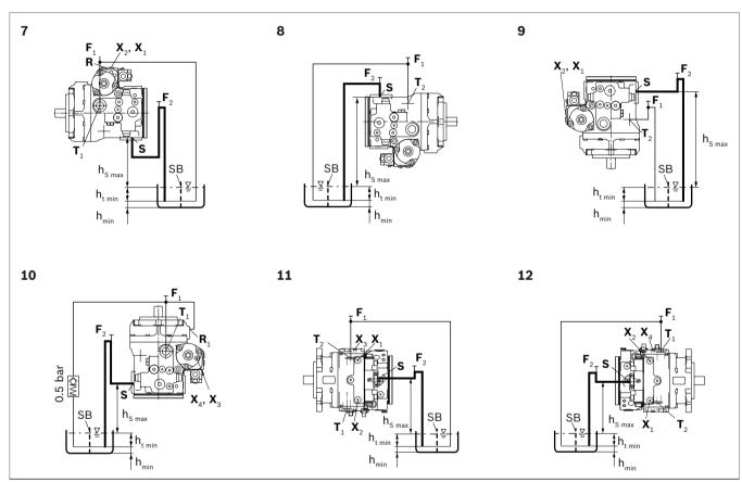
Fig. 9: Above-reservoir installation A4VG with installation position 7-12
