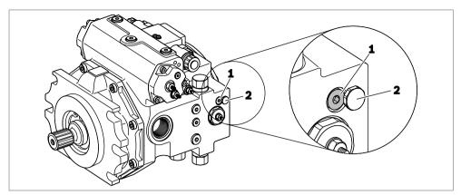
Fig. 3: Activating the bypass function
