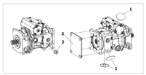
Fig. 1: Axial piston unit
