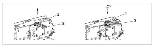
Fig. 12: Changing the lever position of the HW control
