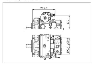
▼ ET - Electric control, direct operated, two DRE
