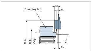
Splined shaft **Z** or **A**The outer diameter of the coupling hub must be smaller than the case diameter **d**, in the area pear the drive shaft
