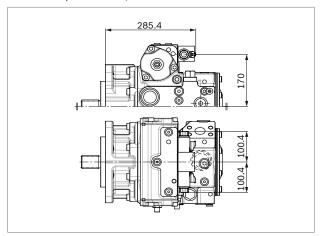
▼ ET - Electric control, direct operated, two DRE
