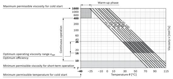
$_{1)}$  The FKM shaft seal is permissible for temperatures of -25 °C to +115 °C, please contact us for temperatures below -25 °C.
