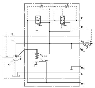
The metering orifice (control block) (1) is not included in the scope of delivery.
