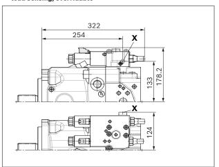
▼ DRS/DRG - Remote-controlled pressure controller, load sensing
