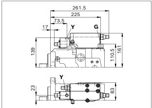
▼ LRDU2 - Power controller, pressure cut-off,
