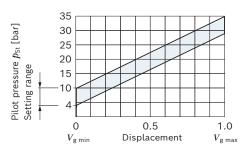
Pilot pressure increase  $V_{\rm g\ min}$  to  $V_{\rm g\ max}$ :  $\Delta p$  = 25 bar
