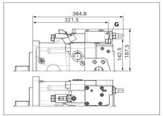
▼ EP2G2 - Electric control with electrically overridable pressure cut-off (positive control)
