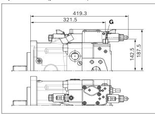
▼ DRS/DRG - Remote-controlled pressure controller, load sensing
