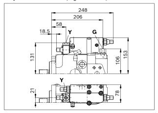
▼ LRDU2 - Power controller, pressure cut-off, hydraulic stroke limiter (positive control)
