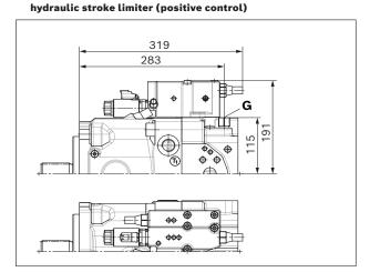
▼ HD2D - Hydraulic, pilot-pressure related control, pressure cut-off
