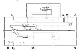
With an external control pressure supply, it is possible for the pump to swivel slightly beyond the zero position (to the mechanical stop).
