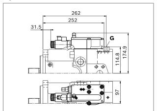
▼ EP2G2/EP2G4 - Electric control with electrically overridable pressure cut-off (positive/negative control)
