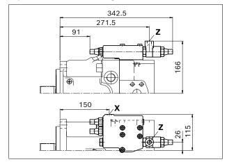
▼ HD2D - Hydraulic, pilot-pressure related control, pressure cut-off
