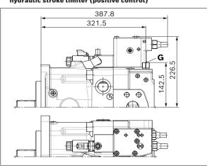
▼ LR3DS - Power controller, high-pressure-dependent override, pressure cut-off, load sensing
