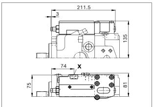
▼ LE2S - Power controller, electrical override, load sensing (negative control)
