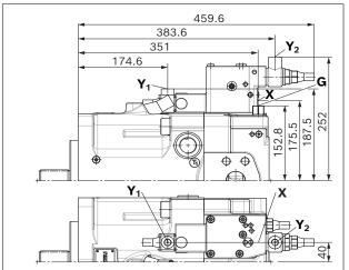
LRDH2 - Power controller, pressure cut-off, hydraulic stroke limiter (positive control)
