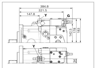
▼ EP2D - Electric control, proportional solenoid, pressure cut-off
