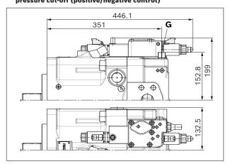
▼ DRL - Pressure controller, parallel operation
