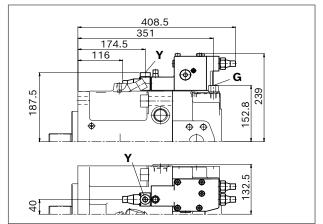
▼ LRDU2 - Power controller, pressure cut-off,
