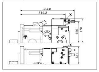
▼ DRL - Pressure controller, parallel operation
