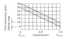
Pilot pressure increase  $V_{\rm g\ max}$  to  $V_{\rm g\ min}$ :  $\Delta p$  = 25 bar
