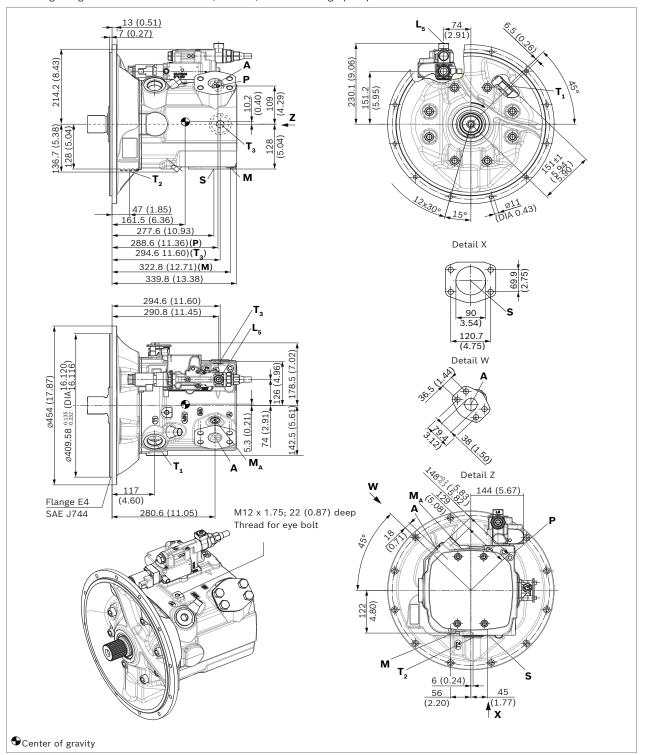
**L5E2 – Power controller with pressure controller, load-sensing and with electric swivel angle sensor** Mounting flange G3 based on SAE J617; 409-12; without charge pump
