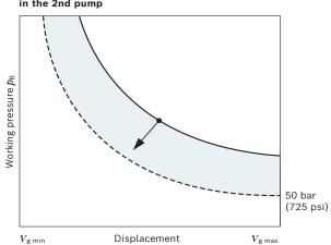
Effect of power override of a pump with increasing pressure in the 2nd pump
