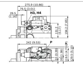
▼ LRDRS0 - Power controller with pressure controller and load-sensing, fixed setting
