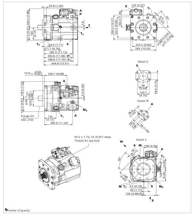
**LRDRS0 – Power controller with pressure controller, load-sensing and with electric swivel angle sensor** Without charge pump, clockwise rotation
