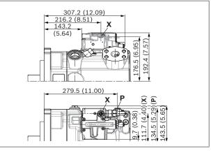
▼ S3/S4 - Load-sensing, internal pressure, electric-proportional
