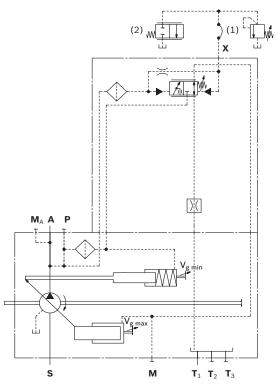
1 Pressure relief valve (not included in the scope of delivery)
