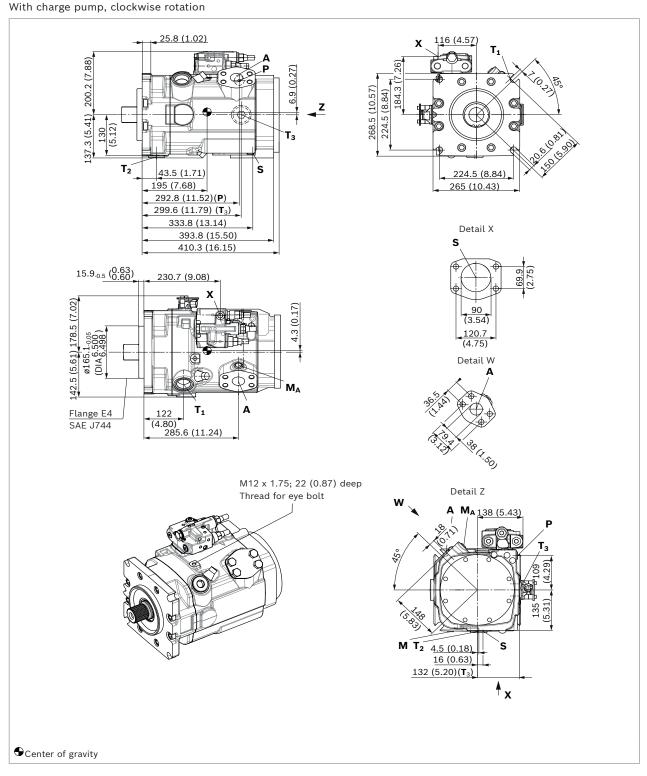
LRDRS0 - Power controller with pressure controller, load-sensing and with electric swivel angle sensor
