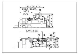
▼ S3/S4 - Load-sensing, internal pressure, electric-proportional
