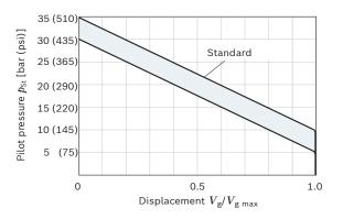
Pilot pressure increase  $V_{\rm g\ max}$  to  $V_{\rm g\ min}$ :  $\Delta p$  = 25 bar (365 psi) When ordering, state in plain text:
