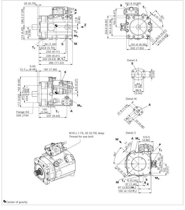
**LRDRS0 – Power controller with pressure controller, load-sensing and with electric swivel angle sensor** Without charge pump, clockwise rotation
