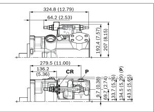
▼ E1/E2; E4 - Stroke control electric-proportional
