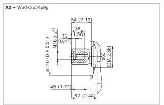
Involute spline according to ANSI B92.1a, 30° pressure angle, flat root, side fit, tolerance class 5
