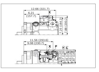
▼ S3/S4 - Load-sensing, internal pressure, electric-proportional
