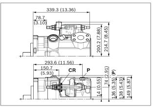
▼ E1/E2; E4 - Stroke control electric-proportional
