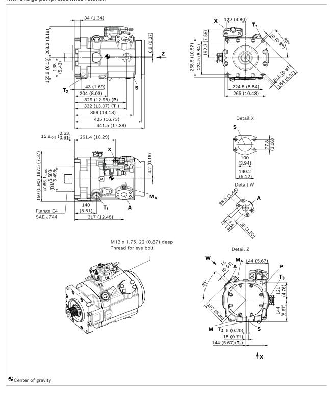
**LRDRS0 – Power controller with pressure controller, load-sensing and with electric swivel angle sensor** With charge pump, clockwise rotation
