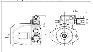
▼ D3/D4 Pressure controller with override, electric-proportional, counter-clockwise rotation
