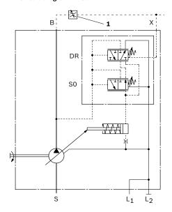
The metering orifice (control block) is not included in the scope of delivery.
