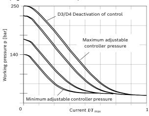
Characteristic curve measured with pump in zero stroke Further information on request.
