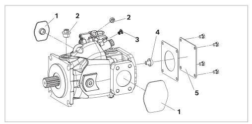
Fig. 1: Axial piston unit A10VOH145 series 60
