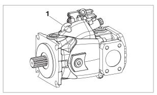
Fig. 4: Transport lug on the housing
