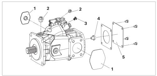
Fig. 9: Removing transport protection
