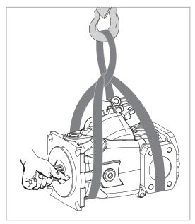
Fig. 5: Transport with lifting strap
