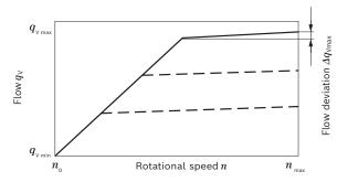
Characteristic curves valid for  $n_1$  = 1500 rpm and  $t_{\rm fluid}$  = 50 °C.
