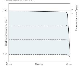
Characteristic curve valid for  $n_1$  = 1500 rpm and  $t_{\rm fluid}$  = 50 °C.
