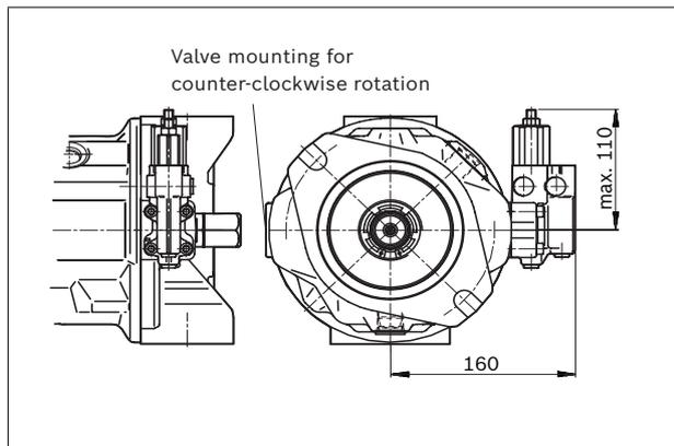
▼ **DRG - Pressure controller, remotely controlled**
