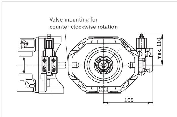
▼ **DRG - Pressure controller, remotely controlled**
