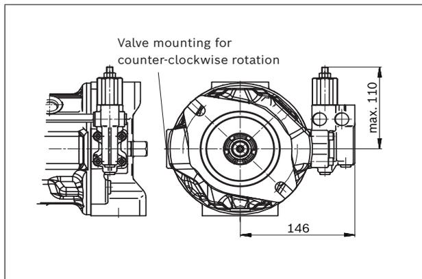
▼ **DRG - Pressure controller, remotely controlled**
