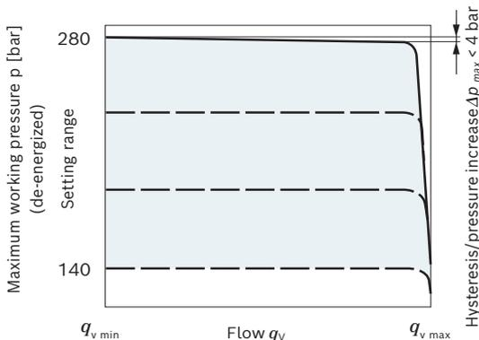
Characteristic curves valid at  $n_1 = 1500$  rpm and  $\vartheta_{fluid} = 50$  °C.
