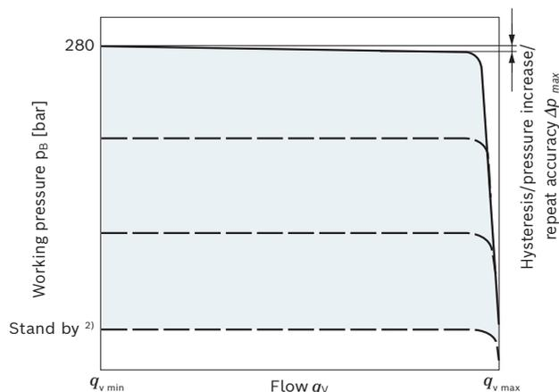
Characteristic curve valid at  $n_1 = 1500$  rpm and  $\vartheta_{fluid} = 50$  °C.
