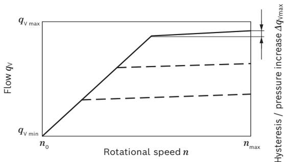
Characteristic curves valid at  $n_1 = 1500 \text{ rpm}$  and  $\vartheta_{\text{fluid}} = 50 \text{ °C}$ .
