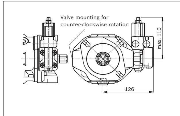
▼ **DRG - Pressure controller, remotely controlled**
