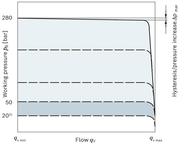
Characteristic curve valid at  $n_1 = 1500 \text{ rpm}$  and  $\vartheta_{\text{fluid}} = 50 \text{ °C}$ .
