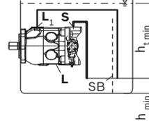
1) Because complete air bleeding and filling are not possible in this position, the pump should be air bled and filled in a horizontal position before installation.
