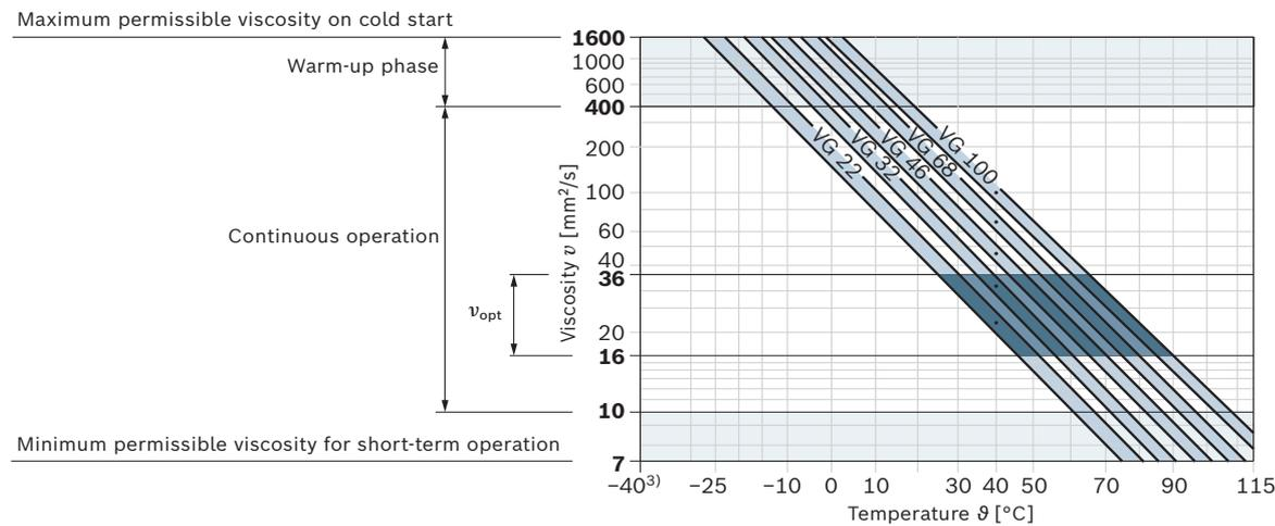
1) This corresponds, for example on the VG 46, to a temperature range of +4 °C to +85 °C (see selection diagram)
