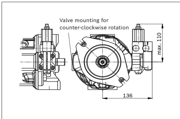
▼ **DRG - Pressure controller, remotely controlled**
