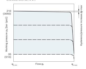
Characteristic curve valid at n1 = 1500 rpm and  $\theta$  fluid = 50 °C (120°F).
