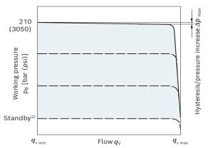
Characteristic curve valid at  $n_1$  = 1500 rpm and  $\vartheta_{fluid}$  = 50 °C (120°F).
