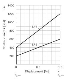
Hysteresis static current-displacement characteristic curve < 5 %.</li>
