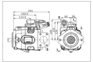
▼ DRF/DRS/DRSC - Pressure and flow controller, series 53
