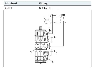
Because complete air bleeding and filling are not possible in this position, the pump should be air bled and filled in a horizontal position before installation.
